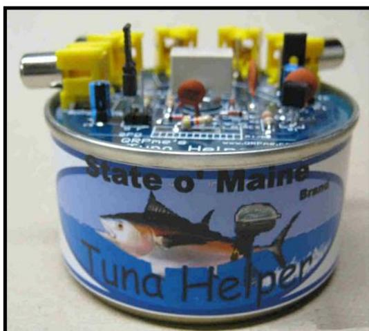
Your Tuna Helper is now ready to automatically switch your antenna between the transmitter and receiver! I use RGB component video cables to hook it up in my station.
